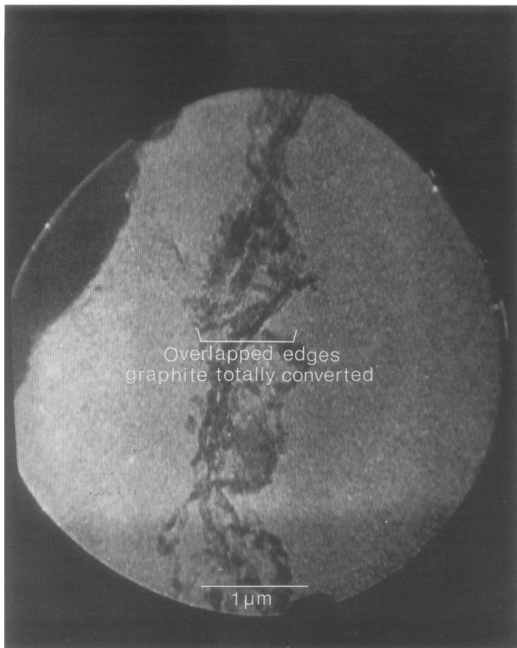
FIG. 8. Final view of the catalyst after all the graphite has been consumed.
